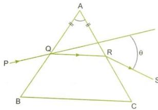
**Q11** Calculate the value of  $\theta$ , for which light incident normally on face AB grazes along the face BC.
